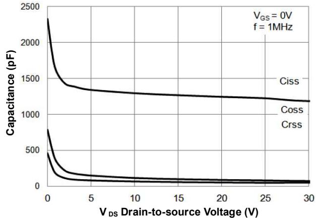
Fig.8 Capacitance Characteristics
