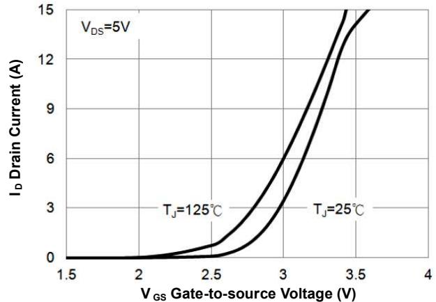
Fig.2 Transfer Characteristics
