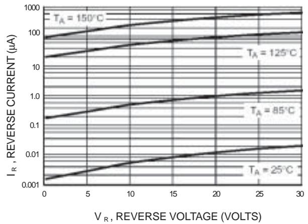
Figure 3. Leakage Current
